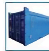
20'x8'x8'6" Open Top 6058 x 2438 x 2591 Gross: 20,000kg Tare: 4,000kg Payload: 16,000kg * PVC Tarpsulin included
