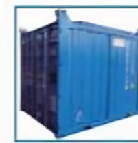
10'x8'x8'6" Open Top 2991 x 2438 x 2591 Gross: 10,000kg Tare: 2,250kg Payload: 7,750kg * PVC Tarpsulin included
